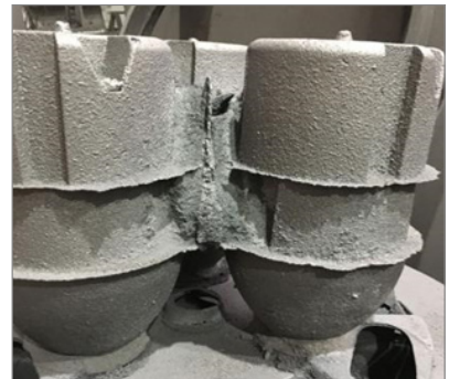
Figure 7: Feeder arrangement – three 6.8 cm modulus feeders
