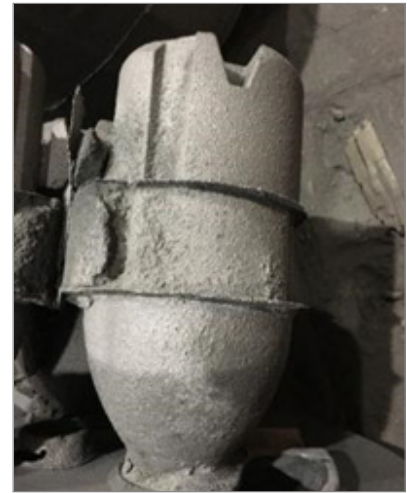
Figure 6: Cast feeder – 6.8 cm modulus
